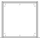
4 Fit the top and bottom track. Fix using track screws
