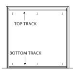
Fix Nylon Guides to top of doors 50mm from the edges using screws provided.
