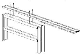
3. Fit and screw closing jamb to track section. With 45mm screws provided
