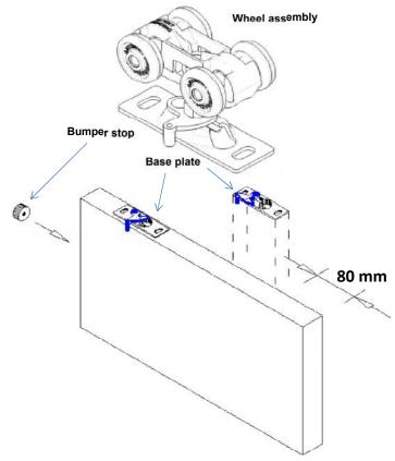
Insert door into cavity unit and tilt up until adjusting bolt of the hanger will slide into the seat of the door plate. Lock into place with nylon lock tabs.
